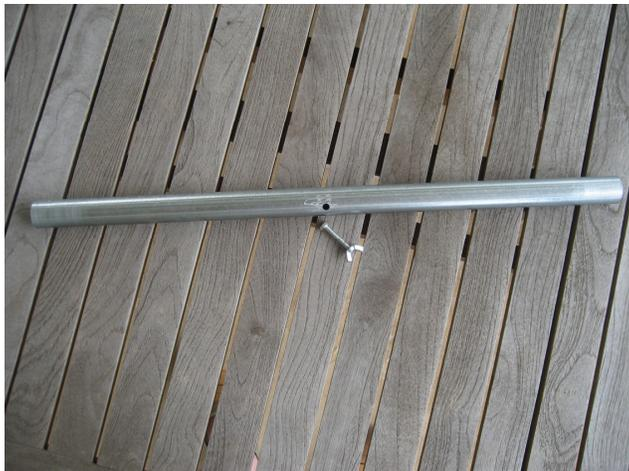
Finish assembly of the tripod by securing the 24" center guide tube pictured left into the center 1" conduit coupling installed on the tripod bracket by tightening the set screw. Install the legs and secure with set screws. Fully assembled the tripod should look like the first photos on the following page.
