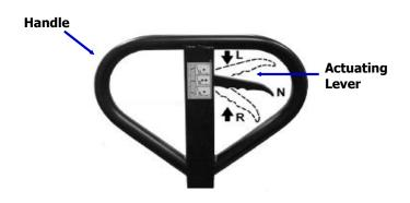
Raise the forks by pushing the actuating lever down (R position on diagram) and pumping the handle up and down. One inch clearance between the floor and pallet is usually sufficient.
