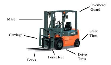
The main parts of a forklift are:
